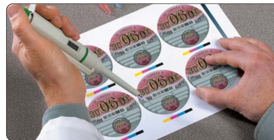
SERRS reagents are applied with a pipette to a 1 to 2mm 2 area of the sample.
