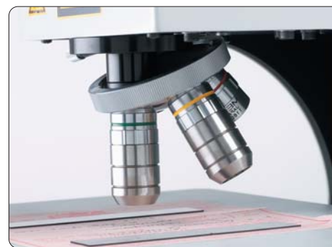
A range of lenses provides on screen magnification of up to x600 on a 22" monitor.
