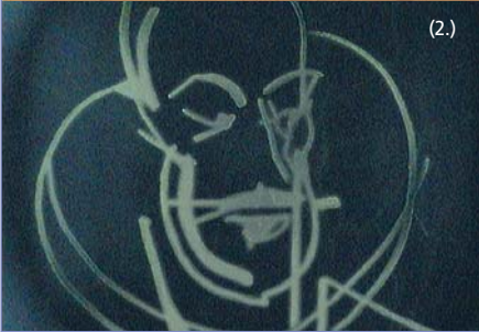
anti-Stokes fluorescent feature within a Portuguese e-passport viewed under normal lighting (1.) and intense infrared lighting (2.).
