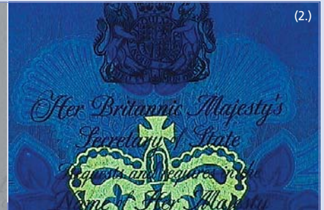
British passport viewed with infrared light (1.) showing variations in the infrared absorption of printed text and also viewed with incident UV lighting (2.) showing fluorescence.
