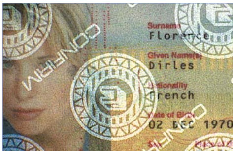
Coaxial lighting reveals retro-reflective patterns on an identity card.
