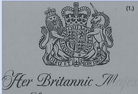
British passport viewed with infrared light (1.) showing variations in the infrared absorption of printed text and also viewed with incident UV lighting (2.) showing fluorescence.
