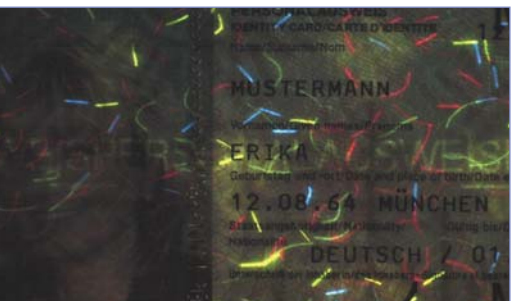
2: shows fluorescent fibres seen using transmitted 365nm UV.
