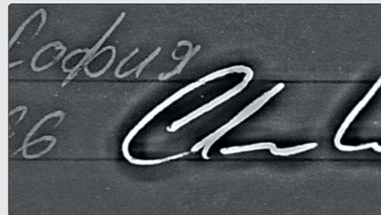
Differences in infrared fluorescence reveals an alteration to a document.
