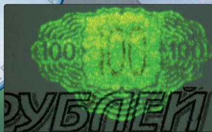
ANTI-STOKES SECURITY FEATURES revealed with high intensity IR lighting.
