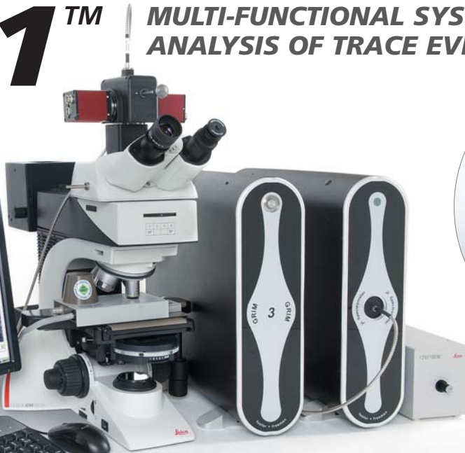
Above: Multiplexer with 5 megapixel CCD camera for image processing and the fibre-optic feed to the micro spectrometer.
