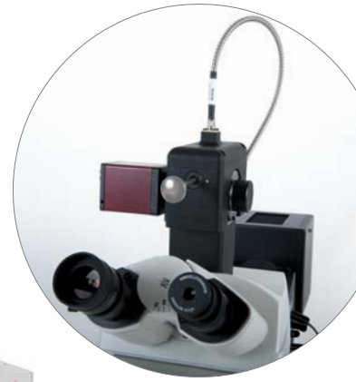
Above: Multiplexer with 5 megapixel CCD camera for image processing and the fibre-optic feed to the micro spectrometer.
