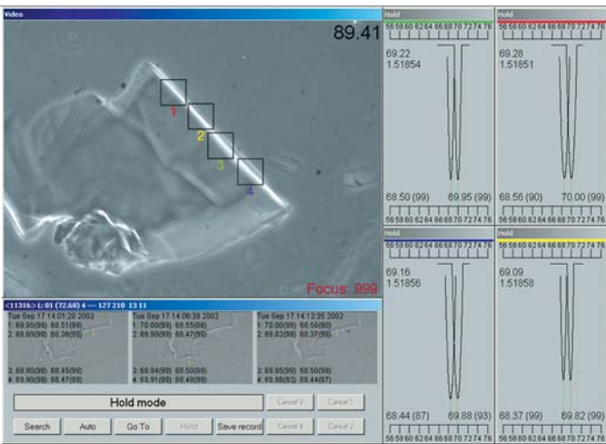
Above: Glass RI measurements using the GRIM3 module
