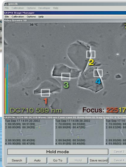
In a motoring offence glass samples from the suspect vehicle are compared to fragments of glass recovered from the victims clothing.
